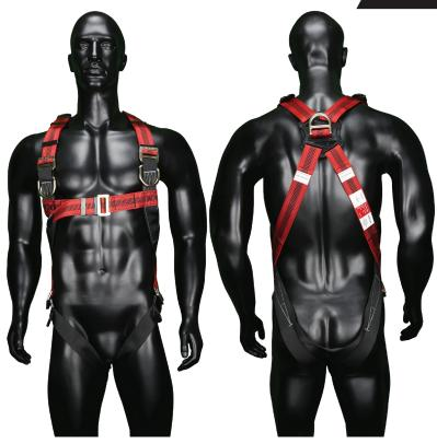
Class L full body harness suitable for work positioning, fall arrest & work restraint situations with one dorsal attachment D-ring, and two chest attachment D-rings. comfort pad at the shoulder waist & thigh enhances the efficiency of workers during long working hours.
