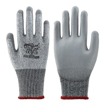
13G high-performance polyethylene (HPPE) liner with a polyurethane (PU) palm coated glove offering Cut level 5 protection.
